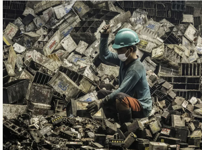
A worker hacks at a used car battery with a machete to remove the lead cells for recycling. Image by Larry Price. Indonesia, 2016.
