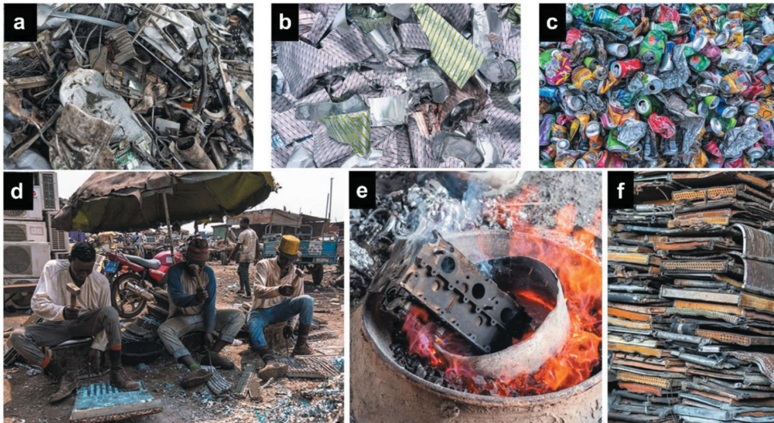
Figure 1. Source materials used to produce the cookware used in this study. (a) Small mixed metals. (b) Plastic-coated blister foils. (c) Aluminum cans. (d) Workers removing aluminum air conditioner fins. (e) Engine block. (f) Auto radiators.
