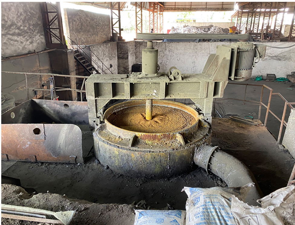
FIGURE 4. Substandard refining kettle as frequently observed in ULAB recycling plants in sub-Saharan Africa
